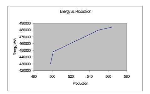
The SEC is varying in the range of 858 to 894 kWh/MT. The SEC has shown a reduction in trend with higher production during April 2004.
